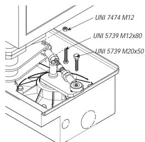
Note: the arms are fitted with several holes to enable different gate-leaf opening angles.
