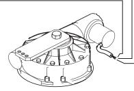
Connection for the **delayed closing** 400V A.C. gearmotor
